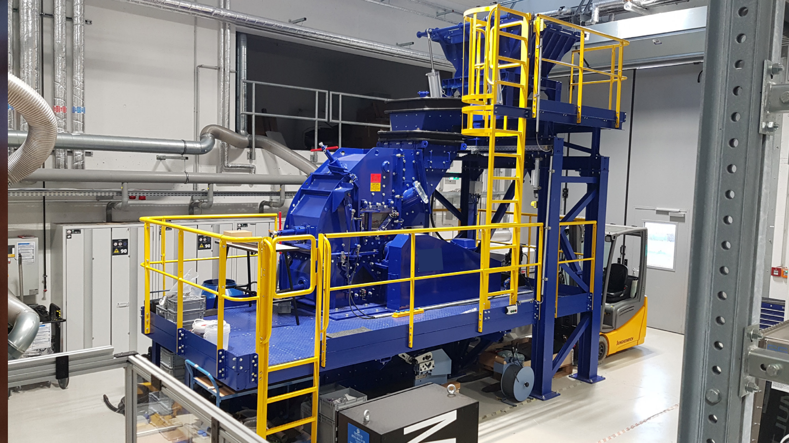
Impact mill/impact crusher for comminution. © Fraunhofer IWKS
